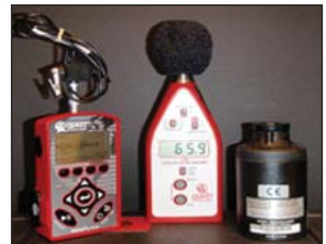
(left to right) Noise Dosimeter, Sound Level Meter, Calibrator
