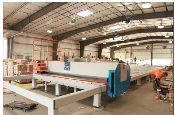
*The gantry is the heart of production, the table layout and pressing system press the preset nail plates into the truss, which increase production and reduces labor injuries.*
