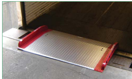
Operators must know the capacity of the equipment used, including dockboards and bridgeplates. Never exceed recommended load capacity.
