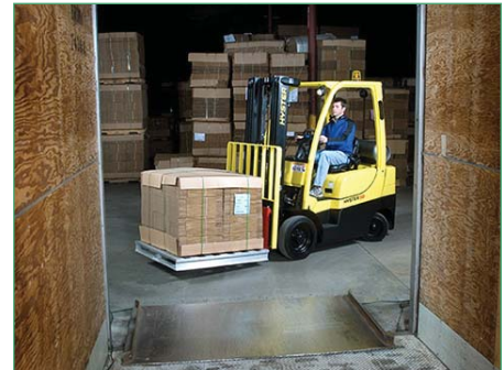
Make sure dockboards or bridgeplates are properly secured; drive over them carefully and slowly and make sure their rated capacity is never exceeded.
