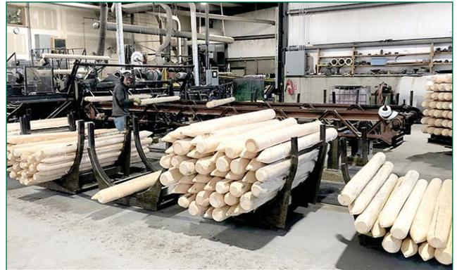
*The process of becoming a post is only partly finished. The posts now go to the preserving process.*
