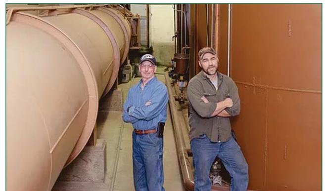
*Preservative treating cylinders where pressure cycles push preservative into dry wood cells. After final vacuum, posts return to drip pad for 7 day fixation period.*
