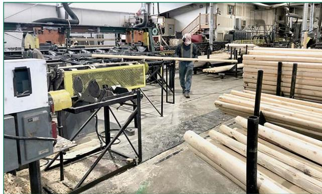
*The pole peeler provides rails that are uniform in size and make a good looking fence.*
