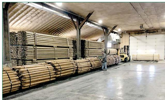
*Completed poles and posts in the drip pad are ready for inspection to confirm that the wood has received the proper treatment before being sent to market.*
