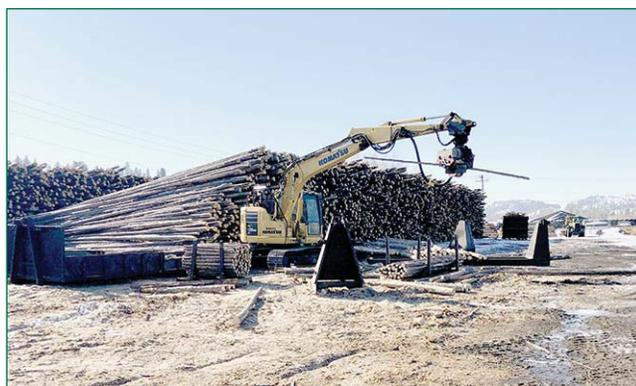
*Here, the operator is cutting raw logs into the appropriate length.*
