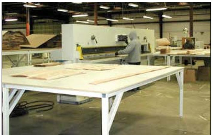
*Veneers are first cut to length then moved to be parallel clipped on one of three guillotines (7', 9' or 14') depending on flitch length.*
