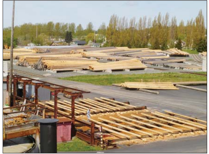
Framing skidway for drying poles before preservative. In the background the poles are in storage.
