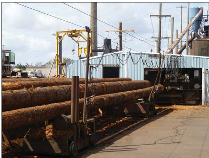
"Barkies" ready to begin processing inside, the peeler will debark the logs and they will be graded.
