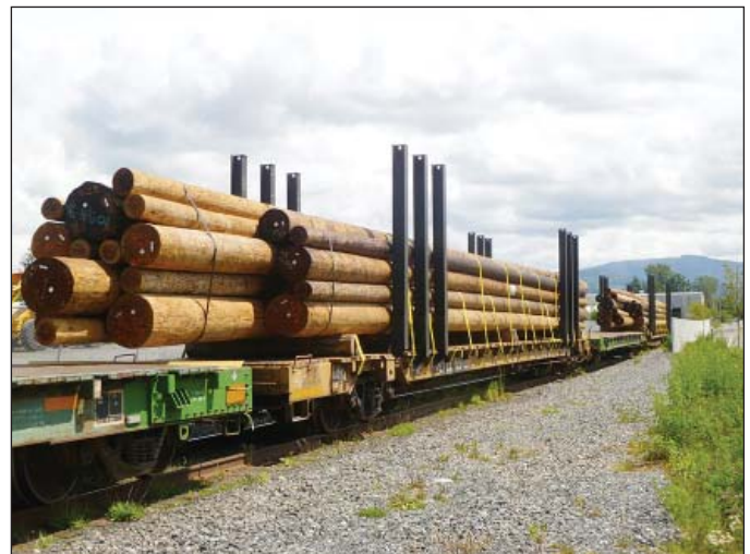
A double overhang load of poles 120 feet long.
