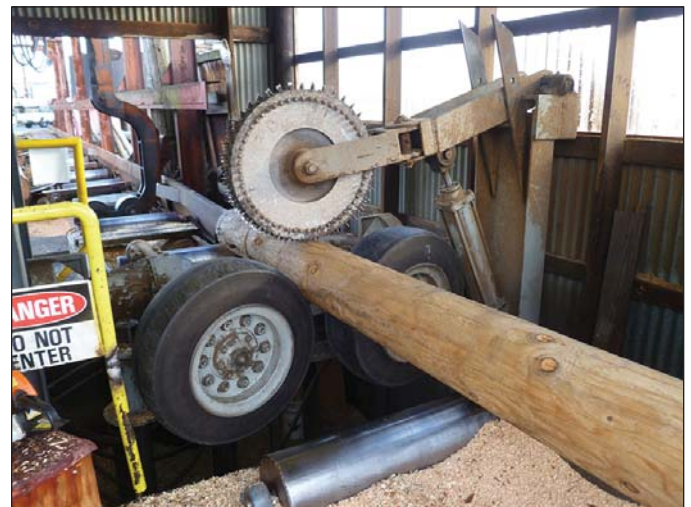
Poles being incised to ensure proper preservative treatment. Notice the teeth that are pushed into the log.
