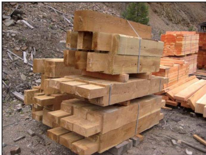
*A bound stack of some of the components for a "four compartment shaft set" for one of the mines.*
