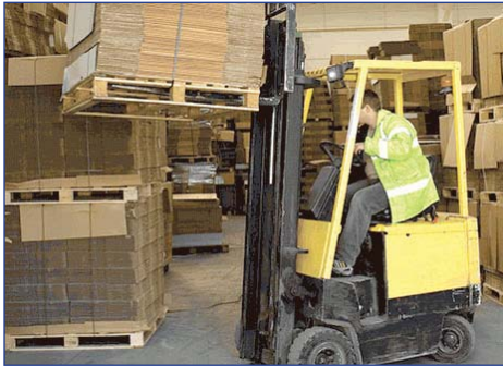
A forklift operator must be trained to drive the forklift. If he is unable to see, he should rearrange the load so vision is not a problem.
