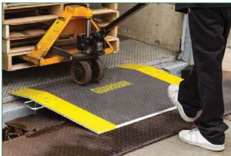
Use all equipment correctly, be sure the dock plate is secure before moving the load.
