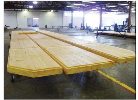
*Glulam beams of Douglas Fir or Red Oak are tongue-and-grooved together with environmentally friendly glues and materials.*
