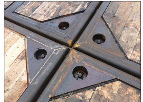
*The links transfer the movement from rig mat to rig mat, which creates a very strong, stable and smooth working platform.*
