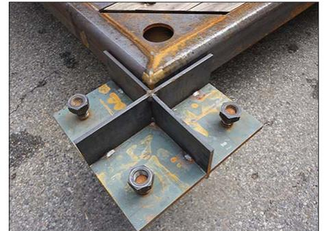
*Crane lifting eyes are built into the corners along with a second generation interlocking linking system that produces linkable platforms.*
