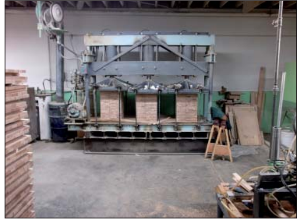
The custom built 50,000 pound hydraulic cold press is loaded with pew ends.
