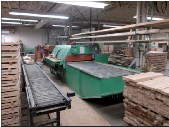
The RF glue machine was custom built and is capable of gluing with a continuous feed for long pews.
