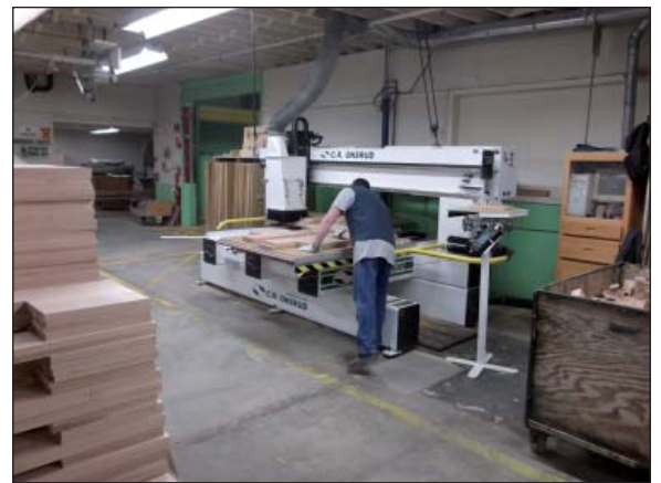
CR Onsrud twin table CNC router loaded with solid oak pew ends.
