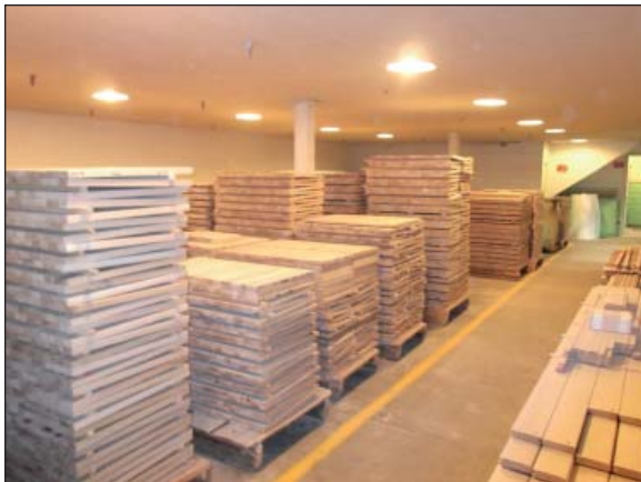
Solid wood panels that have been glued and are curing on stickers.
