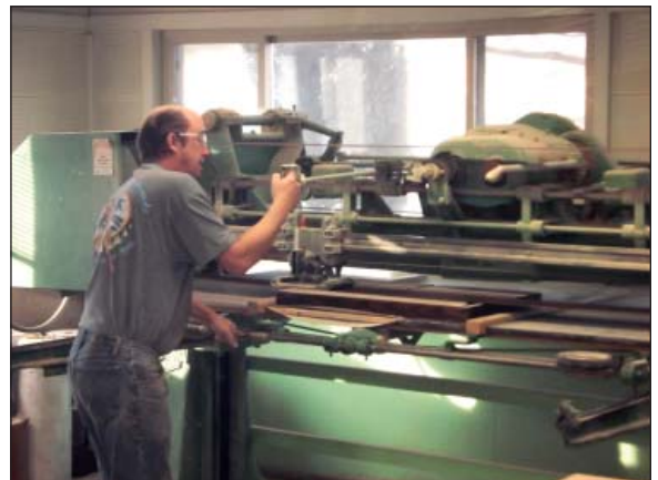
Long time Marshall employee, Robert Cross, stroke sanding a solid oak pew end.
