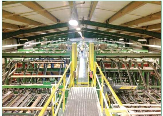
*Inside the sawmill. Dual trimmer sorter stacker lines with the rough on the left and dry on the right.*
