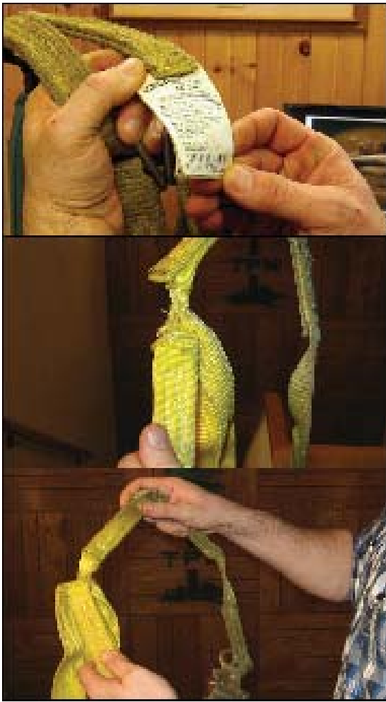
The three photos to the left from top to bottom: Inspect the manufacturers' tag and expiration date. Inspect the harness for excessive wear, cuts or broken fibers. Inspect the stitching points for loose threads or excessive wear.
