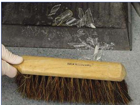
Use a brush and dustpan to pick up broken glass—not a vacuum cleaner.
