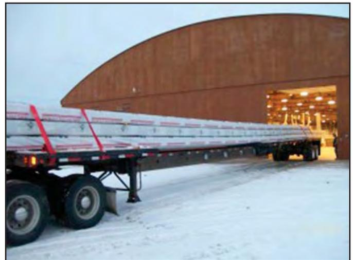
*QB beams are protected with wrapping and can be loaded inside the facility to preserve the surface during transport.*
