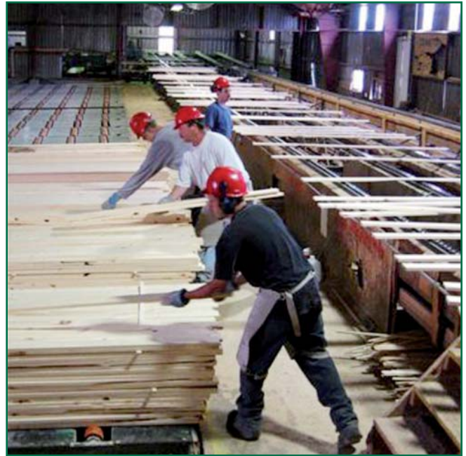
The last stop for a board is the dry chain. Finished lumber is manually stacked into bunks and then steel banded.
