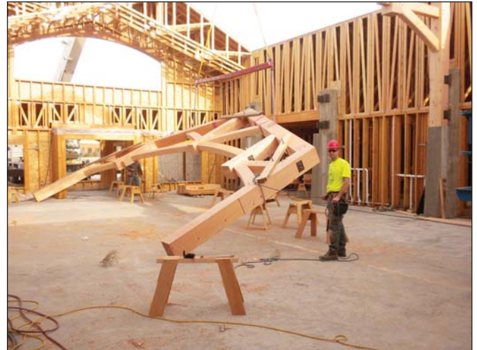
Timber trusses like this are a mainstay of the Marks' product line.
