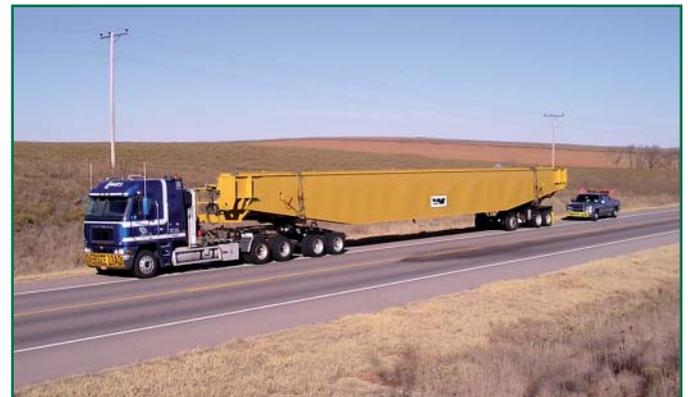
*Oversized load being moved using a steer-trailer set-up.*
