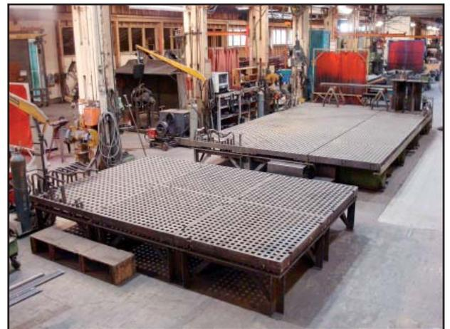
*Kimwood equipment is produced at the fabrication tables.*
