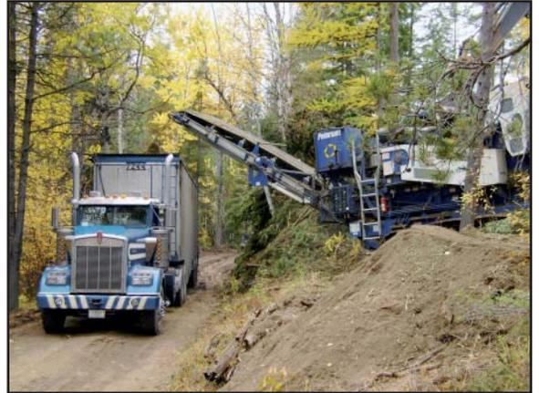
*2410 Peterson Grinder loading Hogfuel into the chip truck from above the haul road.*
