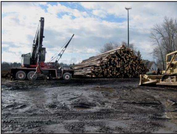
*Prentice log loader unloading logs in the log yard.*
