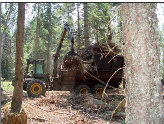
*Jump Trucking's modified brush forwarder used to transfer piles from logging units to roadside.*
