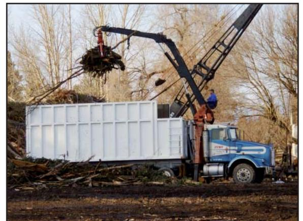
*Jump Trucking's large-capacity brush truck hauling and unloading brush in the collection yard.*
