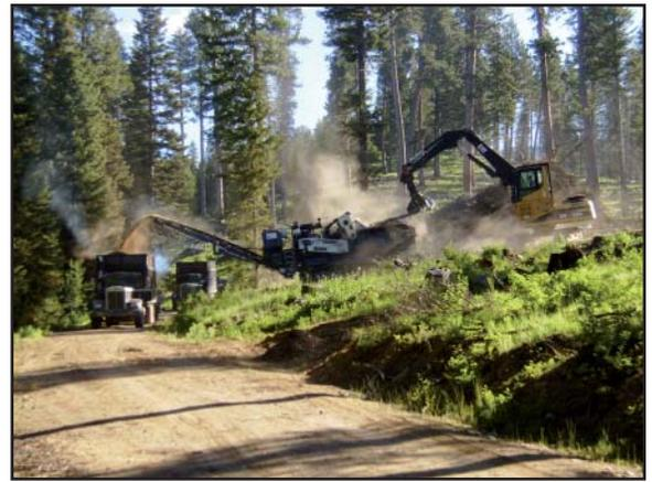
*Jump Trucking's modified Cat loader feeding logging slash into a 2410 Peterson Grinder which is processed and loaded into transfer trucks.*
