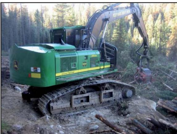
*"Nothing runs like a Deere" A John Deere 2154D Processor, with a Waratah HTH 622B Harvester Head.*
