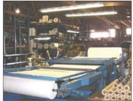
Empire Rubber & Supply Co. can easily slit conveyor belt and other materials up to 72" wide x 1200'+ long using one of our BeltMaster slitting machines.
