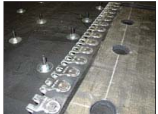
Recessed installation of belt fasteners like the Flexco 550 bolt hinge lace shown and countersunk elevator bolts are available. Empire Rubber can perforate your belt to any pattern you choose.
