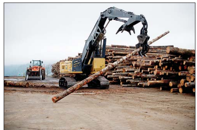
An employee uses the knuckleboom to sort and move logs in the log yard.
