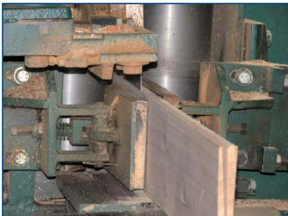
*One of Diebold's 54 inch McDonough Resaws, processing a run of beveled siding.*
