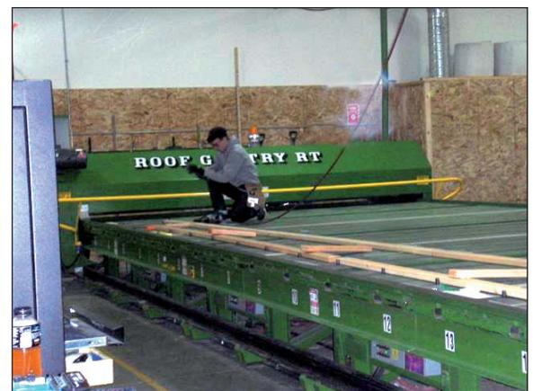
*Employee, Brian Ruby, is kneeling on the truss table in front of the gantry. The gantry rolls across the trusses once the plates are ready and waiting to be affixed.*
