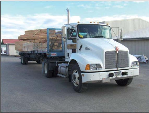
*A load of trusses headed to a building site in the Bitterroot Valley. The truck and trailer set-up can haul a stack of trusses 14 feet in height and up to 70 feet in length.*
