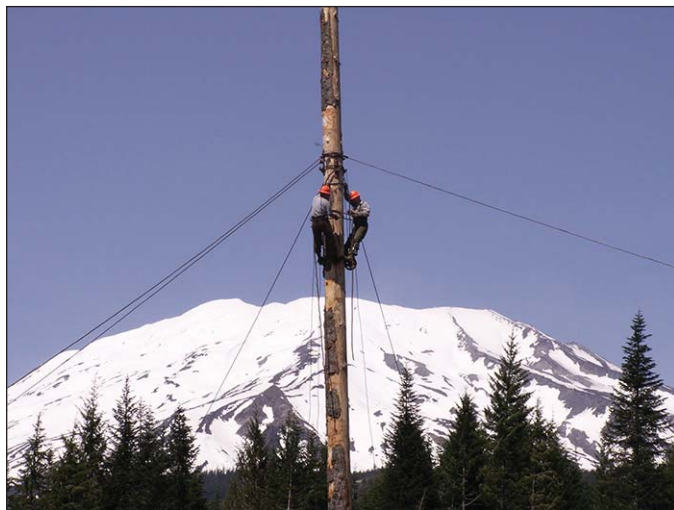
Preparing a spar tree for high-lead logging.
