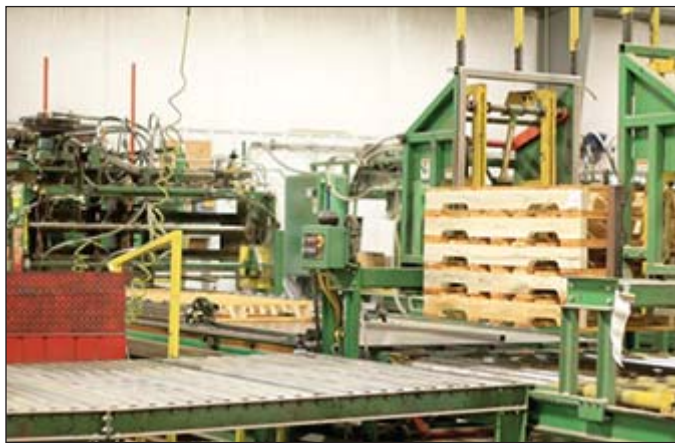
The pallet assembly process begins as each pallet passes through the nailer and down the line for inspection.
