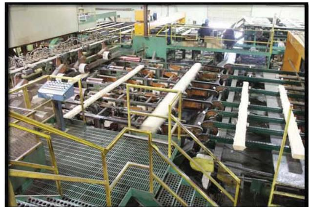
*Cants travel along transfer chains to the optimized cant edger. The edge lazer scans and aligns a cant to a bank of accurately spaced saws to get the most board production from each cant.*
