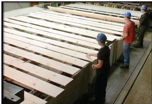
*WWPA-certified graders judge the boards for knot holes, warping, decay, bluestain and other limiting factors in about three seconds per board. After marking the boards, a computer scans and sorts the lumber by grade.*
