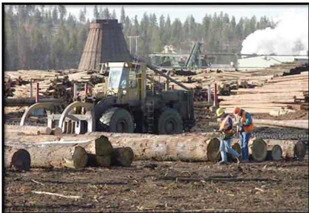
*Bennett's scalers use a "Decimal C" scale stick to measure the diameter and length of each log, then calculate how many boards can be cut from each.*
