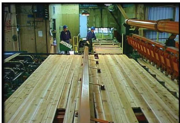
*When a bin is full, it is emptied onto transfer chains where the lumber travels to the stacker.*
