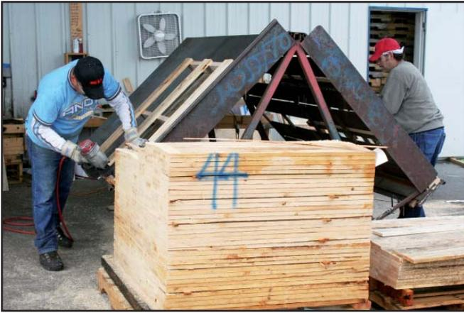
*Eusebio Sanchez (left) nails the bottom boards to a custom-sized pallet, while Jose Leyva-Lopez (right) completes the pallet assembly by nailing the top boards on the pallet utilizing a pallet jig.*
